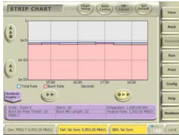
Figure 10: Timeline strip chart of error performance showing bit and burst performance
